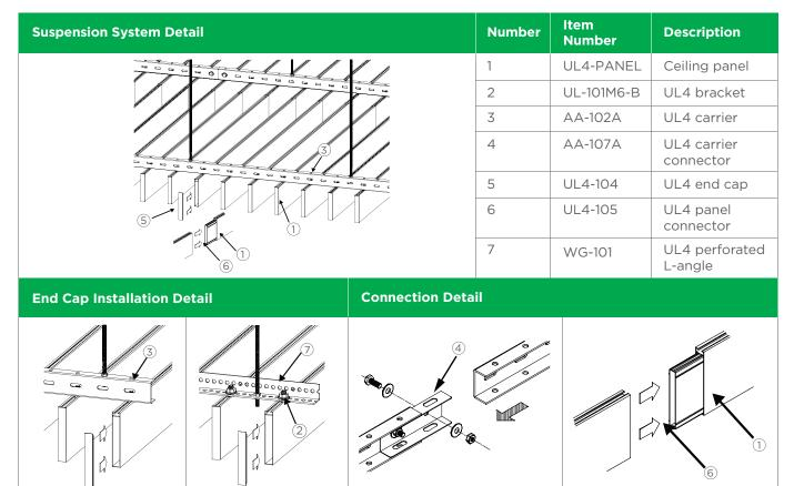
The ceiling is suspended by UL4 carriers (3) and UL4 brackets (2). The distance between each carrier is about 1200mm. The carrier connector (4) is used to connect two carriers for a continuous layout. The carriers are made of galvanised steel.
